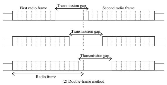
Figure 15: Transmission gap positions with different Nfirst
